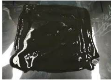
2- The matrix is spread on a plastic film placed on a wooden plate
