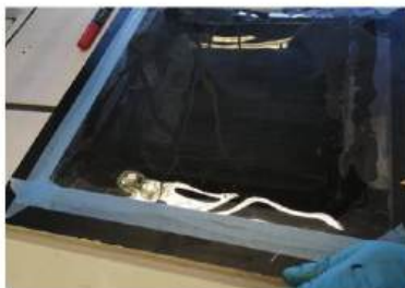
10- The sample is sealed; a force of 50 N is applied on the top. Then, curing is performed at 80 °C for 12 hours.
