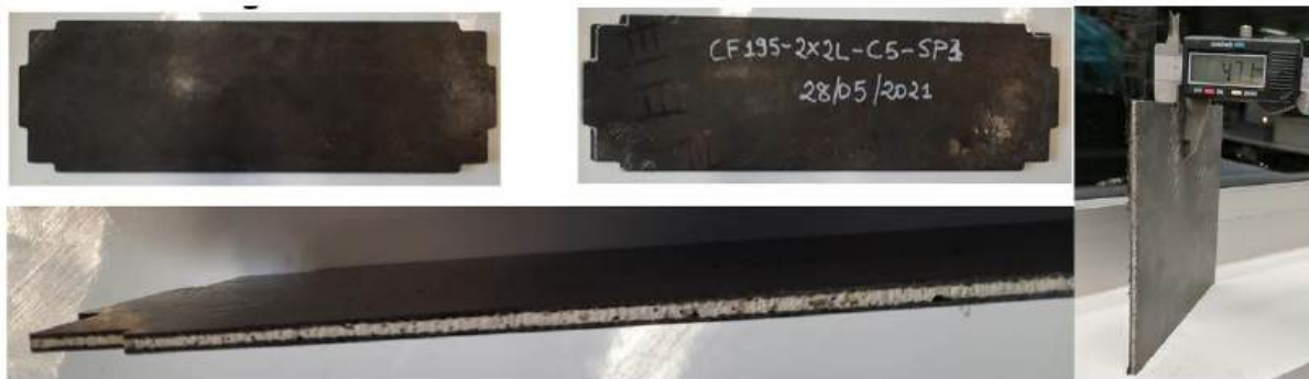
Figure 12. Real scale panels cut in accordance with the design suggested by SPEAR
