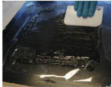
2- The matrix is spread on a plastic film placed on a wooden plate
