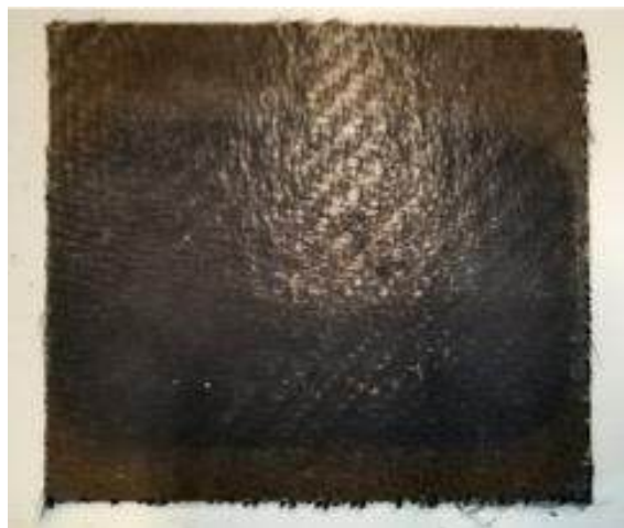
Figure 15 Face of the sample exposed at temperatures above 700 °C; The face of the sample in contact with air outside the kiln remained unchanged.
