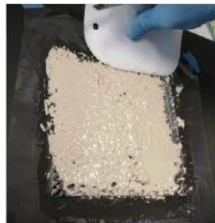
8- The core layer is spread on the top of two impregnated carbon fiber.
